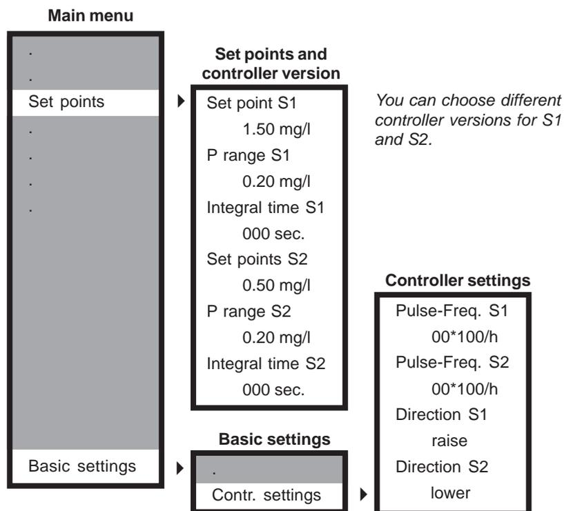
For an impulse-frequency controller you have to set the following parameters:
