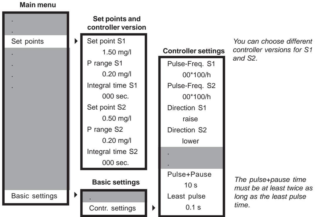
For a pulse-pause controller you have to set the following parameters:
