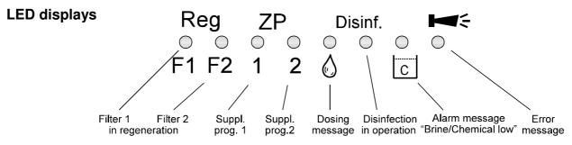
The LEDs display operating statuses, plant functions and pending error messages:
