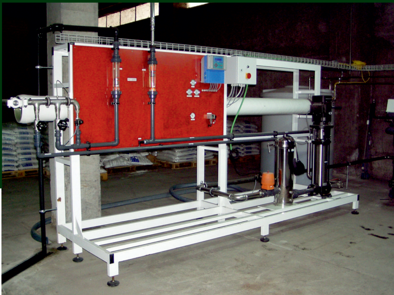
The Softmaster® ROE controls a reverse-osmosis system
