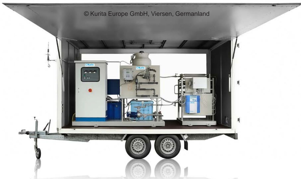
Mobile monitoring system for cooling towers with integrated Testomat 2000® Polymer for monitoring the conditioning agent.
