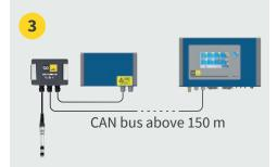
The BlueConnect module also offers the convenient option of providing a power supply for the connected sensor. For extensive measurement networks, the distance between controller and sensor can be increased by installing a BlueConnect. If, in a complex measurement network, the power supply cannot be guaranteed by a single power supply unit, the BlueConnect can supply part of the measurement system with an additional power supply unit.
