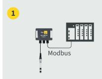
The BlueConnect module effortlessly brings an analogue sensor into the digital world. Once the sensor has been connected, the converted data can be read out via Modbus RTU (RS485). The associated protocol is freely available, enabling a direct connection to a PLC or a Modbus master.
