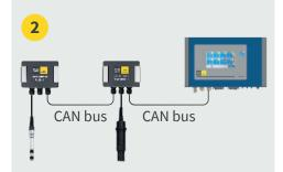
The BlueConnect module enables the cost-efficient integration of an analog sensor into the BlueBox system via CAN bus. If no Modbus interface is available, the module can also be used to connect digital sensors. The Blue-Connect is equipped with three cable connections for simple wiring and further looping of the CAN bus connection. This allows a straightforward set-up of complex measuring systems.
