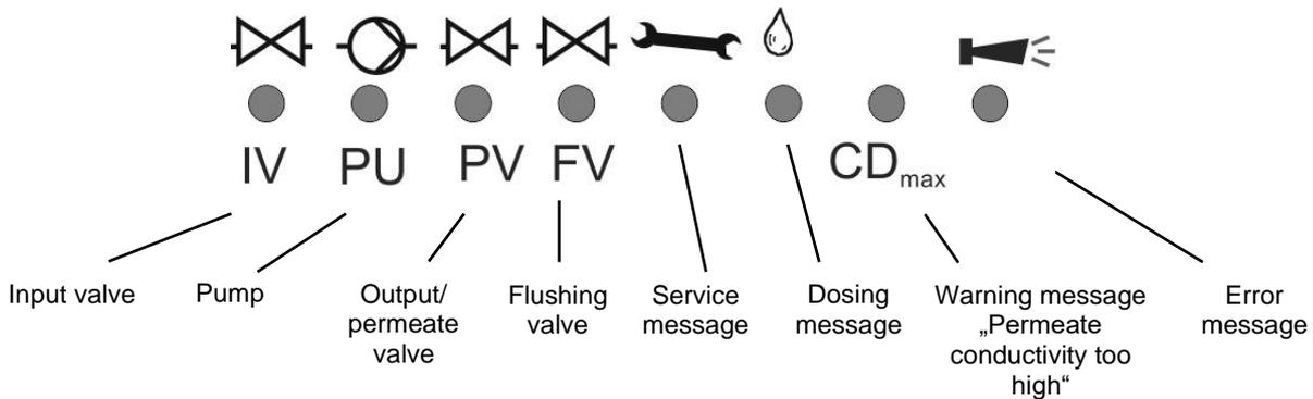
The LEDs display active plant components and occurring error messages.
