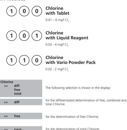
Select the desired determination with the arrow keys [▲] and [▼]. Confirm with [₄] key.
