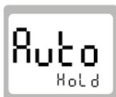
The display shows Auto/HOLD in alternating mode together with the result.
