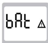
If "bAt" appears in the upper section of the display, this means that the batteries are completely empty.
