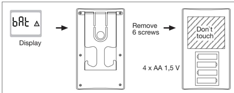
When inserting the batteries, ensure correct polarity!
