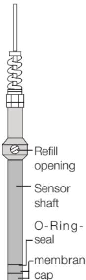
The housing of the sensor probe is made of PVC. With the exception of the sensor shaft, all parts must be serviced regularly and replaced if necessary.
