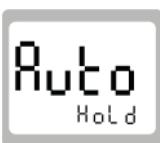
The display shows Auto/Hold in alternating mode together with the result.
